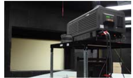
Christie Digital Roadie 25K DLP projectors utilized in a rear-projection configuration power the two main screens in the sanctuary.
