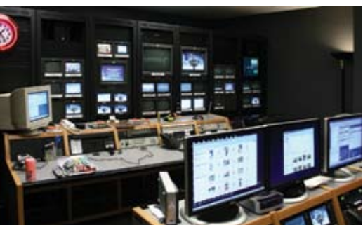
Idlewild's video control room is well equipped with a Ross Video Synergy 2 production switcher and Leitch 32 X 32 SDI and AES3 matrix routers. Idlewild current uses live video for image magnification (IMAG), and has plans to expand into broadcast.
